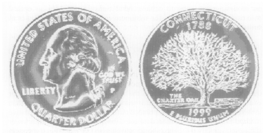
FIG. 15 Image of a coin generated from the sound reflected from the surface in air-coupled (noncontact) mode. The image was produced using an NCA-1000 (SecondWave Systems, Boalsburg) and an NCT230-R6 (3 MHz, 6.4 mm diameter and 6.4 mm focal length) transducer. (Image courtesy of Dr M. Bhardwaj.)
